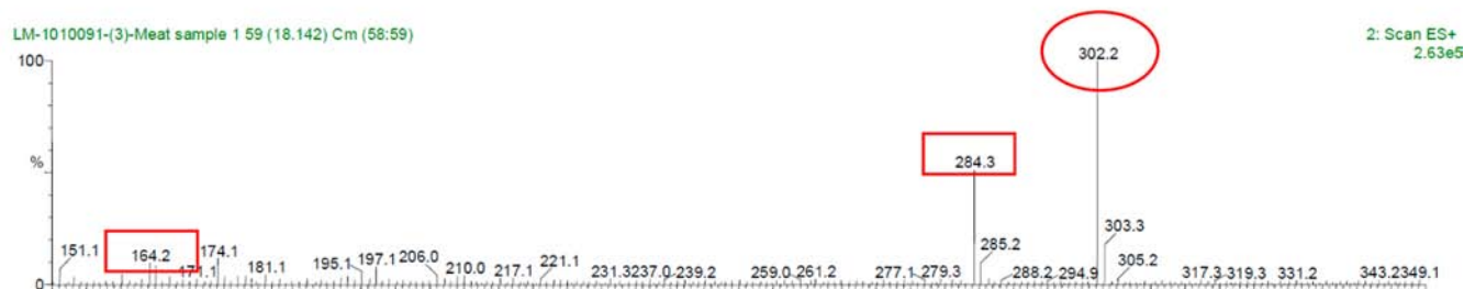
Figure 7. MS spectra of (A) RP standard solution and (B) S7. Column, Zorbax eclipse plus C18 Narrow Bore RR (2.1 × 100 mm, 3.5 μm); mobile phase, 0.1% formic acid in H 2 O and 0.1% formic acid in methanol (50:50); flow rate, 0.2 mL/min; mode, positive electrospray mode; voltage, 3 kV [25 V (cone), 3 V (extractor), and 0.1 V (RF lens)]; source temperature, 98 °C; desolvation temperature, 248 °C; and gas flow rate, 600 L/h in desolvation and 100 L/h in the cone.
