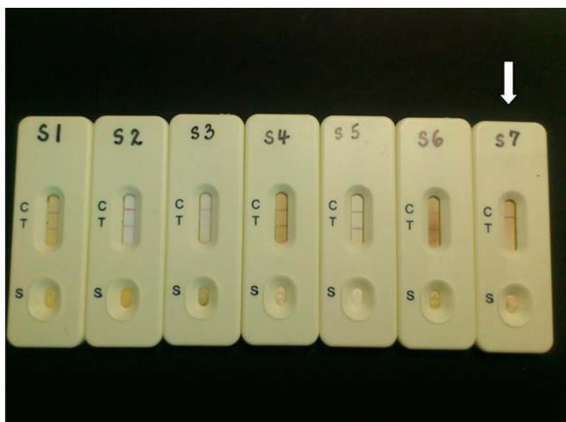
Figure 6. Results for seven real samples using commercial test kits. Two lines represent no RP detected, and one line means that the result is positive.
